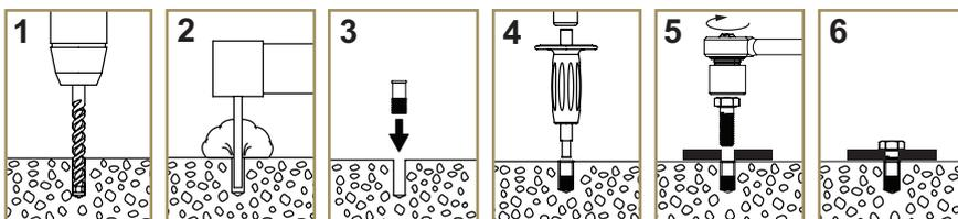
1. Drill the required hole diameter size ( $d_{h=12mm}$ ) using the included drill bits.
