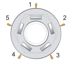
When orange is visible from all bumps, installation and inspection is complete.
