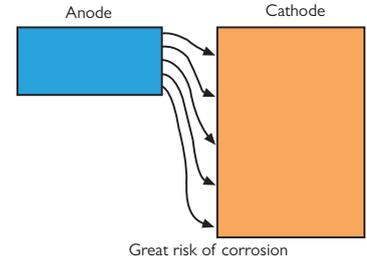
The combination of small anode surface/ large cathode surface therefore involves a greater risk of corrosion.
