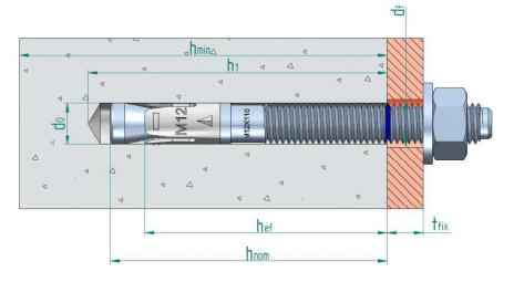
Nominal diameter of drill bit  $d_0$ : d<sub>f</sub>: Fixture clearance hole diameter Effective anchorage depth hef: h<sub>1</sub>: Depth of drilled hole
