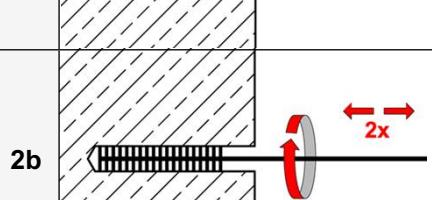
Brush the drill hole **2x** with Cleaning Brush RB (Table B1 or B2). Observe and check brush diameter  $d_b$ . When inserting the brush into the drill hole, a clear resistance must be noticeable. Otherwise use a new Cleaning Brush.
