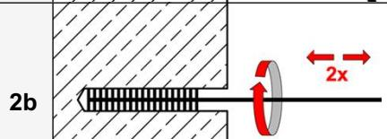
Brush the drill hole **2x** with Cleaning Brush RB (Table B1 or B2). Observe and check brush diameter  $d_b$ . When inserting the brush into the drill hole, a clear resistance must be noticeable. Otherwise use a new Cleaning Brush.
