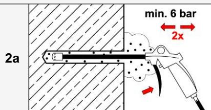
Blow out the drill hole completely at least **2x** from the bottom of the drill hole with compressed air.
