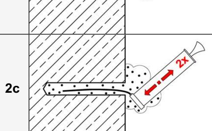
Blow out the drill hole completely at least **2x** from the bottom of the drill hole with blow-out pump.
