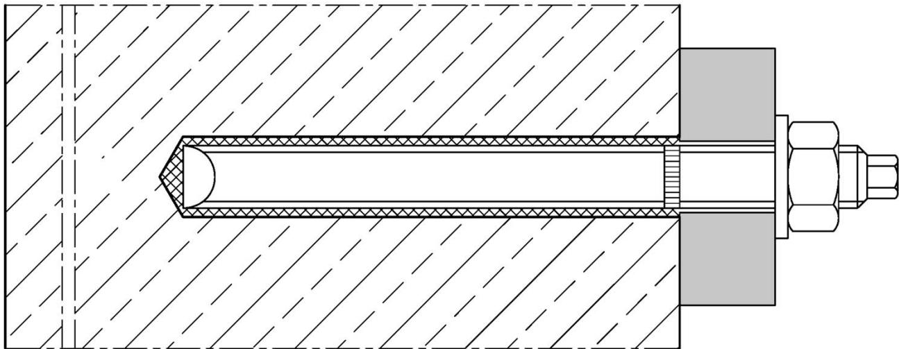
**Installation situation Chemical Anchor VZ with Internally threaded anchor rod VZ-IG<sup>1)</sup>** (optional annular gap filled with mortar)
