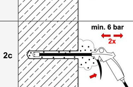
Blow out the drill hole completely at least **2x** from the bottom of the drill hole with compressed air.
