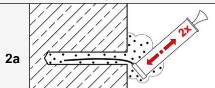
Blow out the drill hole completely at least **2x** from the bottom of the drill hole with blow-out pump.
