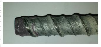
process becomes very hard and in most cases, does not drive-in at all. On the other side of the hardness spectrum, it cannot be too hard because of the possibility of the brittle chipping off of the thread during the driving process. This balance in material strength and hardness must be established in conjunction with the thread pitch and profile.
