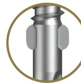
Wings assist in producing a clearance hole in timber. Wings break off once the screw starts to drill through the metal.
