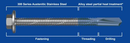
A Bi-Metallic screw, is comprised of two metal types. The point is manufactured from high carbon steel that is heat treated to give it the ability to self-drill. The head section is manufactured from a corrosion resistant stainless steel (304 or 316). The two metals are "fused together" to form a screw that offers excellent self-drilling properties, combined with exceptional corrosion resistance.
