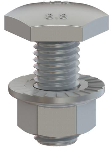
A Hobson 8.8 Fascia Bolt assembly consists of a property class 8.8 bolt and a class 8 nut. They come in two types of coating, zinc plated (ZP) and hot dip galvanised (HDG).
