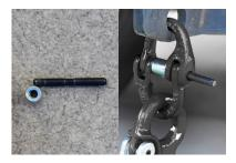
**Step 3.** Bring the two halves of the links together and partially insert locking pin to hold the parts together.
