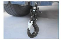
**Step 4.** Insert the locking collar with the recessed side facing the pin and push the pin in until it holds the collar in place.
