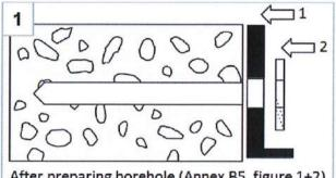
After preparing borehole (Annex B5, figure 1+2), position first fixture (1), than filling washer (2)
