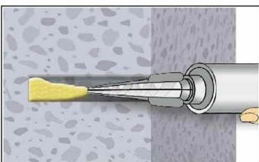
6. Starting from the bottom or back of the cleaned anchor hole, fill the hole up to approximately two-thirds with adhesive. Slowly withdraw the static mixing nozzle as the hole fills to avoid creating air pockets. If the bottom or back of the anchor hole is not reached, an appropriate extension nozzle must be used. Observe the gel-/ working times given in Table B5.
