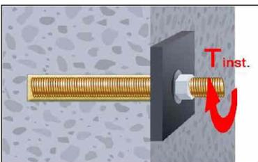
13. After full curing, the add-on part can be installed with up to the max. torque (Table B1 or B3) by using a calibrated torque wrench. In case of prepositioned installation the annular gab between anchor and fixture can be optional filled with mortar. Therefor substitute the washer by the filling washer and connect the mixer reduction nozzle to the tip of the mixer. The annular gap is filled with mortar, when mortar oozes out of the washer.
