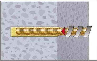
9. Push the fixing element into the anchor hole while turning slightly to ensure positive distribution of the adhesive until the embedment mark has reached the surface level.
