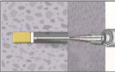
8. Insert piston plug to back of the hole and inject adhesive. If the bottom or back of the anchor hole is not reached, an appropriate extension nozzle must be used.
