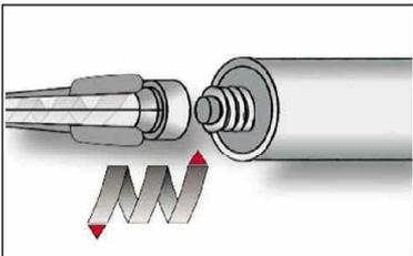
3. Attach the supplied static-mixing nozzle to the cartridge and load the cartridge into the correct dispensing tool. For every working interruption longer than the recommended working time (Table B5 as well as for new cartridges, a new static-mixer shall be used.
