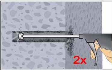
2f. Finally blow the hole clean again with compressed air (min. 6 bar) (Annex B 4) a minimum of two times until return air stream is free of noticeable dust. If the bore hole ground is not reached an extension shall be used.
