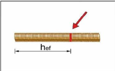
4. Prior to inserting the anchor rod into the filled bore hole, the position of the embedment depth shall be marked on the anchor rods.
