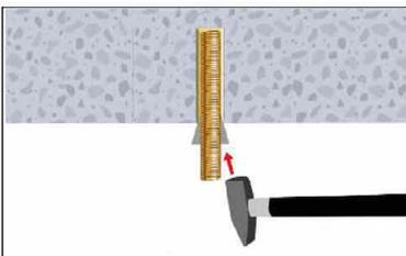
11. For overhead application the anchor rod shall be fixed (e.g. wedges) until the mortar has started to harden.
