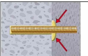
10. After inserting the anchor, the annular gab between anchor rod and concrete, in case of a push through installation additionally also the fixture, must be complete filled with mortar. If excess mortar is not visible at the top of the hole, the requirement is not fulfilled and the application has to be renewed.
