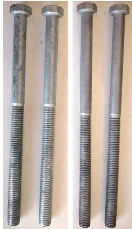
**Figure 2:** Bottom Bolt with the previous shinier finish compared to the current darker and flatter look on the top 3 bolts.
