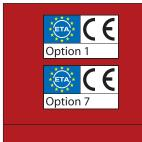
The most common options you find in most published ETA's are **Option 1** (cracked and non-cracked concrete with a range of concrete strengths loaded in various directions) and **Option 7** (non-cracked concrete with a range of concrete strengths loaded in various directions).
